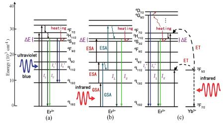
Fig. 3 The mechanism of optical thermal sensing through (a)  $Er^{3+}$  down-conversion under ultraviolet (blue) excitation, (b)  $Er^{3+}$  up-conversion under infrared excitation, and (c)  $Yb^{3+}-Er^{3+}$  energy transfer under infrared excitation.
