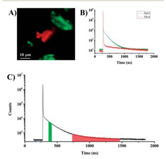
Fig. 4 (A)  $100 \times 100$  pixels photon arrival time image (PArTI) of silica particles dyed with either Nd.1 (green) or Yb.1 (red). Total integrations time 1000 s. (B) Time resolved emission profiles of Nd.1 (green) and Yb.1 (red) extracted from the photon stream. (C) Full time-resolved emission profile recorded by TCSPC while imaging. The red, blue, and green arrival time intervals are selected to generate the best photon arrival time resolved image.
