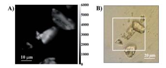
Fig. 2 (A) 100  $\times$  100 pixel total intensity image of a random mixture of silica particles dyed with either Yb.1 or Nd.1. Total integrations time 1000 s. (B) Optical transmission image of the same sample, the white square marks the 60  $\times$  60  $\mu$ m scanning area. The intensity image displays the number of photons that were detected in each pixel.
