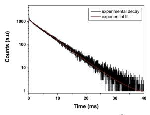
Fig. 8 Photoluminescence decay profile of LaPO<sub>4</sub>:Eu<sup>3+</sup> (0.5 mol%) at emission and excitation wavelength of 593 and 256 nm, respectively.
