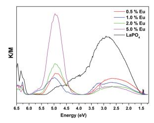
Fig. 15 UV-Vis absorption-energy curves of LaPO<sub>4</sub> and La<sub>1-x</sub>Eu<sub>x</sub>PO<sub>4</sub>.
