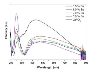
Fig. 14 UV-Vis diffuse reflectance spectra of LaPO<sub>4</sub> and La<sub>1-x</sub>Eu<sub>x</sub>PO<sub>4</sub>
