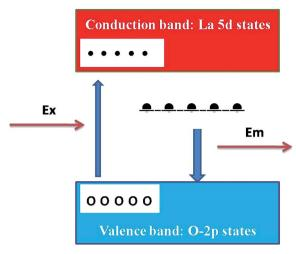
Fig. 5 Schematic model of probable mechanisms responsible for observed emission in LaPO4. In the schematic model, the upper (red) and the lower (light blue) bands are La 5d conduction bands and O 2p valence bands, respectively. The black bar below the conduction band corresponds to the defect level created by the oxygen deficiency. White and black circles correspond to excited holes and electrons, respectively.
