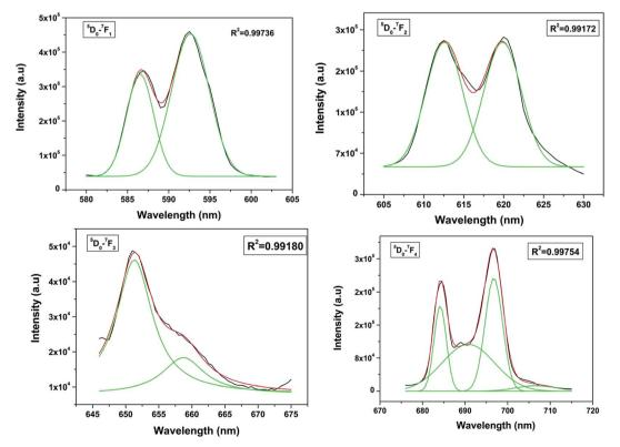
Fig. 7 Stark splitting pattern of europium emission in lanthanum phosphate nanoparticles.
