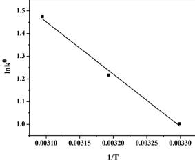
Fig. 11 Plot of  $\ln k^0$  versus 1/T for estimation of thermodynamic parameters for the adsorption of  $Cr(v_i)$  on zinc-biochar (volume: 50 mL; adsorbent dose: 0.1 g; initial  $Cr(v_i)$  concentration: 25, 50, 75, 100, 200, 250, 400, 500 mg  $L^{-1}$ ; pH: 2.0; contact time: 24 h).
