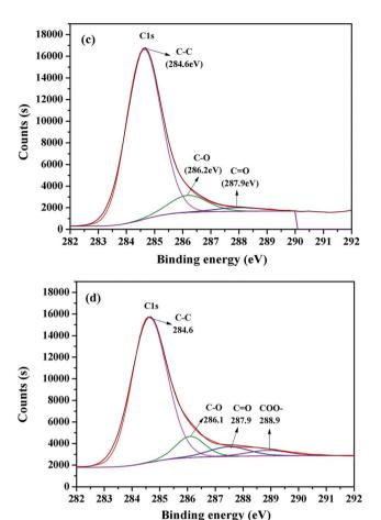
C 1s XPS spectra of biochar (c) before and (d) after modification.
