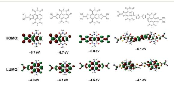
Fig. 2 Frontier molecular orbitals and HOMO/LUMO levels of N,N'-bis(methyl)-substituted model molecules of 1, 2, 3 and 4 estimated by DFT calculations
