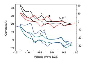
Fig. 4 Cyclic voltammograms of compounds 1, 2, 3 and 4 with 0.1 M  $Bu_4NPF_6$  in dichloromethane solution under a scan rate of 50 mV s<sup>-1</sup>.
