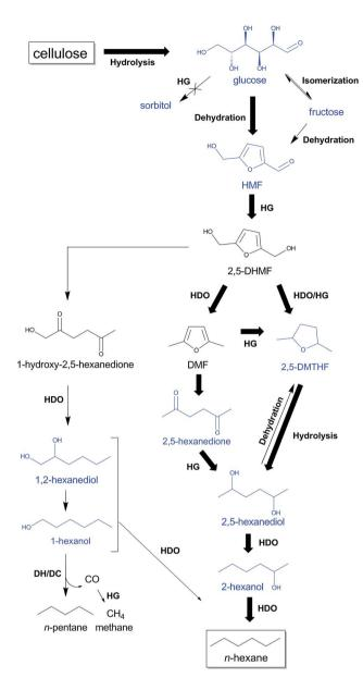
Scheme 3 Proposed reaction pathways from cellulose to *n*-hexane and *n*-pentane through HMF with TSA and htTSA(2)Ru/C, partially based on Liu *et al.*,<sup>88</sup> Alamillo *et al.*,<sup>67</sup> Li *et al.*<sup>60</sup> and Yang *et al.*<sup>92</sup> Intermediates tested in this study are indicated in blue. The most selective reaction pathway from cellulose to *n*-hexane is indicated with bold arrows. HDO, hydrodeoxygenation; HG, hydrogenation; DH/DC, dehydrogenation/decarbonylation.
