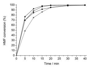
Fig. 2 HMF hydrogenation with Ru/C (gray, ■), htRu/C (black, ●), htTSA(2)Ru/C (black, ▲) and htTSA(135)Ru/C (black, ▼). Reaction conditions: 5.56 mmol HMF, 0.25 g Ru/C (content in the different catalysts), 50 ml H<sub>2</sub>O, 5 MPa H<sub>2</sub>, 333 K.
