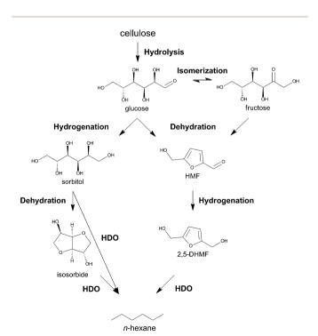
**Scheme 2** Two different pathways for the selective one-pot conversion of cellulose to *n*-hexane: the established sorbitol route (left hand-side) and the here proposed HMF route (right hand-side). Abbreviations: HDO, hydrodeoxygenation. 2,5-DHMF, 2,5-dihydroxymethylfuran.
