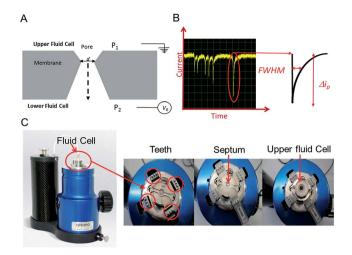
**Fig. 1** (A) Sectional schematic of a pore. The sample is typically placed into the upper fluid cell. (B) Example of baseline current and "blockade" events (current dips) that are each caused by an analyte traversing the pore. Each event is analysed for full width half maximum (FWHM) duration and  $\Delta i_{\rm p}$ . (C) The Izon qNano instrument, showing the fluid cell, teeth and crucifix plastic membrane with aperture.
