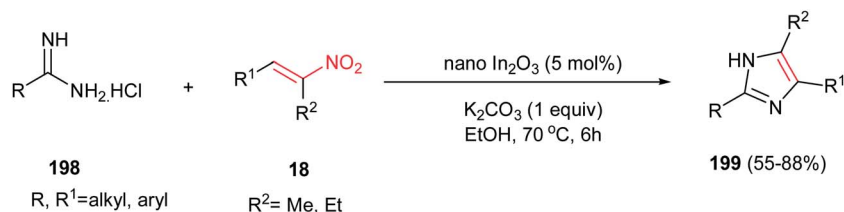
Scheme 67 Synthesis of imidazoles via tandem cyclization between amidine and nitroolefins.
