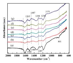
Fig. 4 FT-IR spectra of (a) PANI/CFs with 10 wt% PANI, PANI/CFs after treated with  $Cr(v_1)$  solution for (b) 5, (c) 10, (d) 20, (e) 30, (f) 45 and (g) 60 min, respectively.
