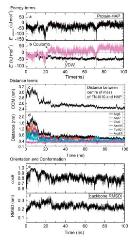
Fig. 6 Time evolution of energy terms, distance terms, orientation, and structure terms. (a) Interactions between protein and HAP; (b) electrostatic and VDW potential energy; (c) distance between COM of FN-III10 and HAP along z-axis direction; (d) residue—HAP distance; (e) orientation (cos  $\theta$ ); (f) backbone RMSD.
