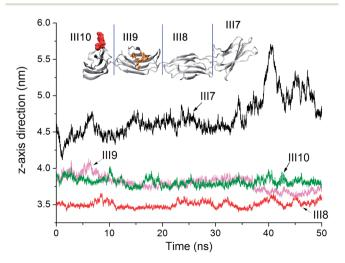
Fig. 10 Time evolutions of the distance between COM of modules and HAP along z-axis direction for modules III7–10 in the FN-III7–10 system.
