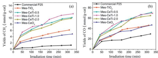
Fig. 18 The yield of CH<sub>4</sub> (a) and CO (b) as a function of the irradiation time over all photocatalysts. Reproduced with permission from ref. 287. Copyright 2013, Elsevier.
