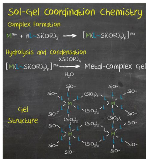
Fig. 9 Sol-gel coordination chemistry, an approach developed for the synthesis of hybrid mesoporous materials through the *in situ* incorporation of chemical functionalities into the framework of silica and organosilica porous materials. Reprinted with permission from ref. 8. Copyright 2013, Wiley-VCH.
