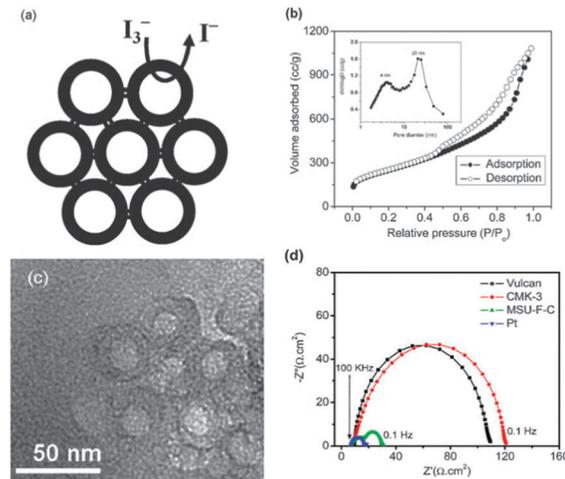
Fig. 22 (a) A schematic illustration of the facile diffusion and reduction of I<sub>3</sub><sup>-</sup> ions in MSU-F-C carbon. (b) The N<sub>2</sub> isotherm and pore size distribution (inset) of MSU-F-C carbon. (c) High-resolution TEM image of microtomed MSU-F-C carbon. (d) Nyquist plots of various carbon electrodes and conventional Pt electrodes in a thin layer symmetric cell configuration. Reproduced from ref. 333. Copyright 2010, RSC.
