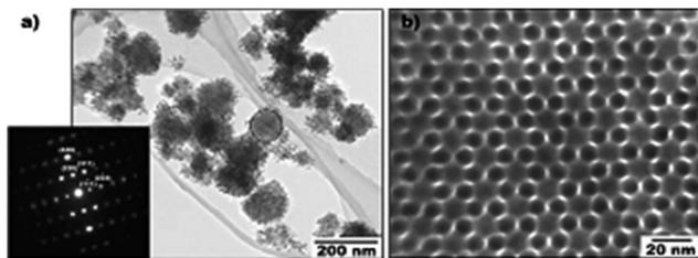
Fig. 7 TEM images at low (a) and high (b) magnifications of KIT-6 mesoporous  $\text{Co}_3\text{O}_4$ , showing highly ordered mesopores. The inset is the corresponding SAED pattern of the circled zone. Reprinted with permission from ref. 72. Copyright 2010, Wiley-VCH.
