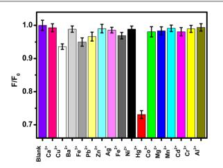
**Fig. 6** Relative fluorescence intensity ( $F/F_0$ ) of the FNCPs in phosphate solutions (25 mM, pH 7.4) with 50  $\mu$ M different metal ions. F and  $F_0$  correspond to the fluorescence intensity of the FNCPs with and without 50  $\mu$ M of different metal ions.
