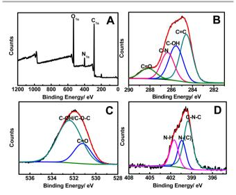
**Fig. 3** The XPS (A),  $C_{1s}$  (B),  $O_{1s}$  (C), and  $N_{1s}$  (D) spectra of the as-obtained FNCPs.
