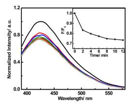
**Fig. 5** Time-dependent fluorescence responses of the FNCPs to 50  $\mu$ M Hg<sup>2+</sup>. Inset shows the *F/F*<sub>0</sub> plotted against time in the presence of 50  $\mu$ M Hg<sup>2+</sup>, where *F* and *F*<sub>0</sub> are the fluorescence intensity of the FNCPs at 427 nm with and without Hg<sup>2+</sup>, respectively.
