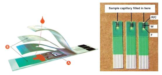
Fig. 4 Cross section of a commercial strip for self-testing of blood glucose (left, reprinted with permission from ref. 26, copyright 2008, American Chemistry Society) and the test strips designed in 2008 (right, reprinted with permission from ref. 225, copyright 2009, Elsevier).
