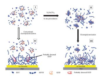
**Fig. 3** Procedures for immobilization of GOx *via* the chemical preoxidation electropolymerization and conventional electropolymerization protocols. Reprinted with permission from ref. 160, copyright 2008, American Chemistry Society.
