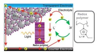
Fig. 8 Scheme of a dye sensitized solar cell.
