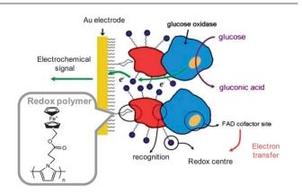
Fig. 9 Scheme of a glucose electrochemical biosensor.
