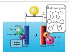
Fig. 7 Scheme of an enzyme-based biofuel cell.
