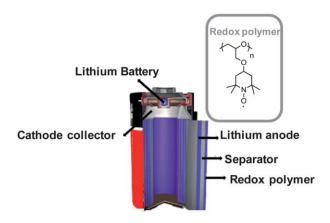
Fig. 5 Scheme of nitroxide organic radical/lithium metal batteries.
