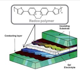
Fig. 10 Schematic representation of an electrochromic device.
