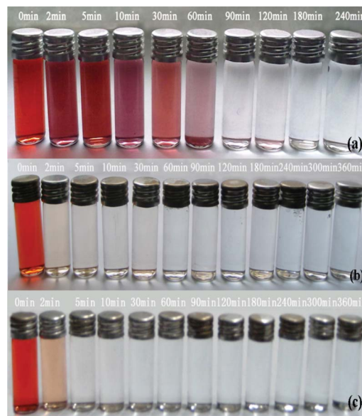
Fig. 6 Photographs of CR solutions (CRS) before and after treatment with CeO 2 at different time intervals: (a) CRS (100 mg L -1 , 50 mL) in the presence of 250 mg of CeO 2 nanoparticles, (b) CRS (50 mg L -1 , 50 mL) in the presence of 20 mg of CeO 2 nanorods, and (c) CRS (80 mg L -1 , 50 mL) in the presence of 150 mg of the CeO 2 mixture of nanoparticles and nanorods.
