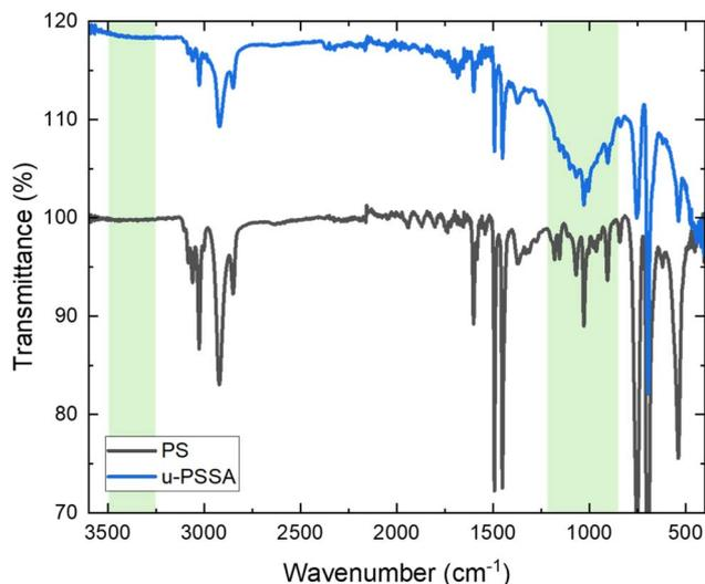
Fig. 1 Spectra of a waste expanded PS and u-PSSA showing a new O–H stretching band at  $3370\text{ cm}^{-1}$  from the sulfonic acid functional group and sulfonate stretch bands between  $950$  and  $1200\text{ cm}^{-1}$ . The new bands are highlighted in green. Note that the u-PSSA spectrum was offset by 20% on the y-axis for clarity.
