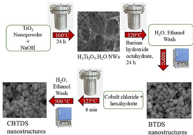
Scheme 1 Schematic of the steps involved in forming \text{H}_2\text{Ti}_2\text{O}_5\cdot\text{H}_2\text{O} nanowires and \text{BaTiO}_3 and \text{CoBaTiO}_3 doughnut nanostructures.
