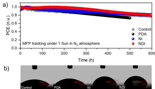
Fig. 6 Operational stability of inverted perovskite solar cell devices. (a) Maximum power point tracking evolution of the unencapsulated device under full solar illumination (AM 1.5 G,  $100 \text{ mW cm}^{-2}$  under nitrogen). (b) Contact angle measurements with a water droplet for the films.
