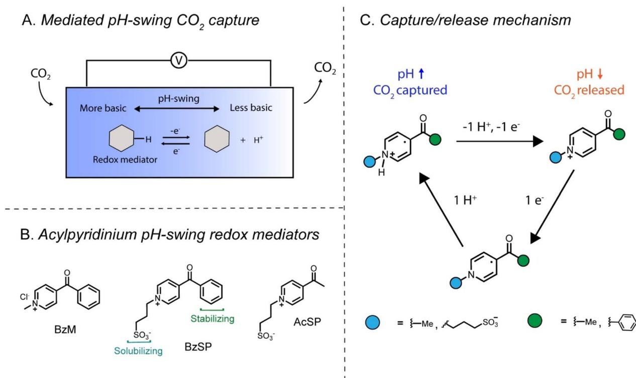
Fig. 1 (A) General scheme for redox-mediated pH-swing carbon capture in one compartment. (B) Acylpyridinium redox mediators used in this work. (C) Mechanism of CO<sub>2</sub> capture with pyridinium mediators.
