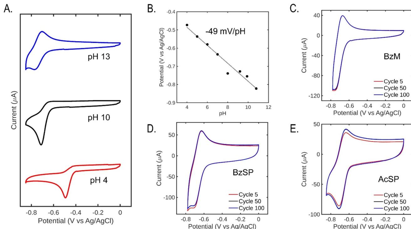
Fig. 2 Cyclic voltammetry of 5 mM pyridinium mediators at 100 mV s<sup>-1</sup> under argon. (A) Cyclic voltammograms of BzM in various buffers with 1 M KNO<sub>3</sub>. (B) Pourbaix diagram of BzM. (C–E) Long-term cyclic voltammograms in unbuffered 1 M KNO<sub>3</sub> of BzM, BzSP, and AcSP.
