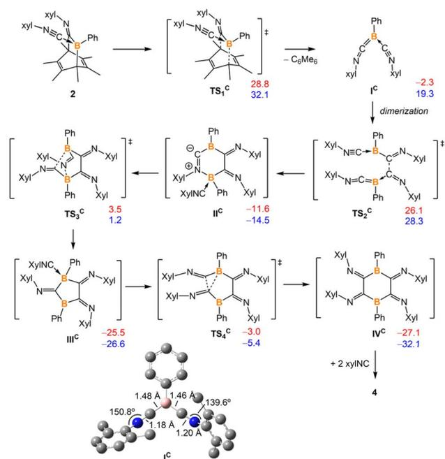
Fig. 4 Energy profiles were calculated for the reaction of **2** to **4**. The relative Gibbs free energies (in red) and electronic energies (in blue) are calculated at 298 K and given in kcal mol<sup>-1</sup>. The calculation is at MO6-2X-D3/6-311g\*\* level of theory with applied solvation models in toluene.
