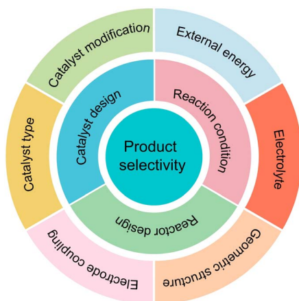
Fig. 6 The factors affecting product selectivity: catalyst design, reaction conditions, and reactor design.
