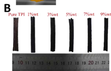
Fig. 7 (A) Geometry of PLA/CB 3D-printed electrodes. (B) Samples of pure TPI and CNTs-TPI 1, 3, 5, 7, 9wt% bars. 76 Copyright, Elsevier B.V.
