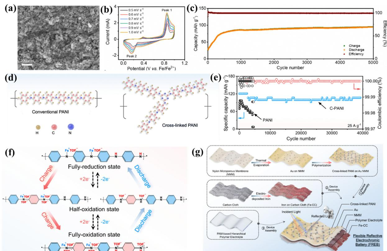
Fig. 8 (a) SEM image of PANI. (b) CV plot at different scan rates. (c) Capacity and CE vs. cycle number at  $0.2 \text{ A g}^{-1}$ .<sup>99</sup> (d) schematic of conventional PANI and C-PANI. (e) GCD cycling performance of PANI vs. C-PANI in aqueous electrolyte. (f) Schematic of the charge storage mechanism *via* C-PANI. (g) Synthesis schematic of FREBs.<sup>108</sup>
