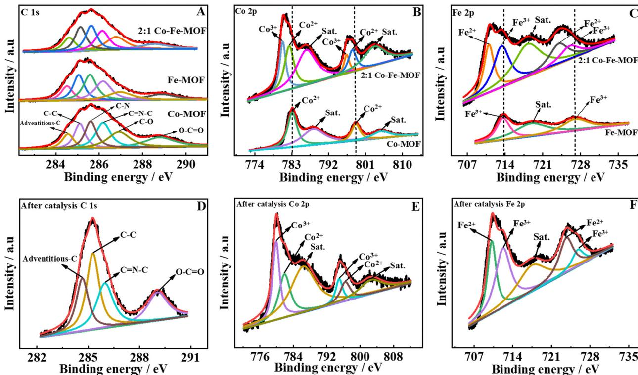
Fig. 2 High-resolution deconvoluted XPS spectra of C 1s, Co 2p, and Fe 2p of the Co-MOF, Fe-MOF, and 2 : 1 Co-Fe-MOF (A)–(C) and after the OER catalysis of the 2 : 1 Co-Fe-MOF (D)–(F).
