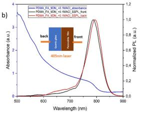
Fig. 2 The crystallography and phase distribution of quasi-2D perovskites (PDMA)(FA)<sub>4</sub>Pb<sub>5</sub>I<sub>16</sub>. (a) Powder X-ray diffractograms of δ-phase and α-phase perovskites made from different precursor solution inks and processing methods. (b) UV-vis absorption spectra and steady-state photoluminescence from both front (perovskite) and back (substrate) sides of the quasi-2D perovskite thin films with  $\langle n \rangle = 5$ . The inset shows the illumination directions.
