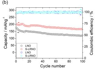
Fig. 5 (a) Initial charge—discharge curves of LNO and S-LRNO synthesised by the solid state method between 2 and 4.3 V at 25 mA g $^{-1}$  (after the formation cycle). (b) The cycling performance of LNO and S-LRNO at 25 mA g $^{-1}$ .
