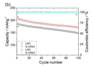
Fig. 7 (a) Initial charge-discharge curves LNO and S-LRNO synthesised by the co-precipitation route between 2 and 4.3 V at 25 mA  $\mbox{g}^{-1}$  (after the formation cycle). (b) The cycling performance of LNO and S-LRNO at 100 mA g<sup>-1</sup>
