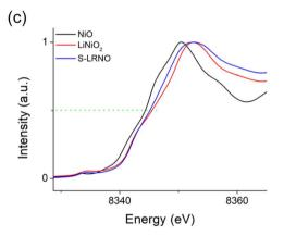
Fig. 2 (a) XRD patterns of Li $_{11}$ Ni $_{0.85}$ O $_2$ , Li $_{1.1}$ Ni $_{0.875}$ S $_{0.025}$ O $_{2-x}$  and Li $_{1.1}$ Ni $_{0.85}$ S $_{0.05}$ O $_{2-x}$  (solid state synthesis route). (b) Observed, calculated and difference profiles from structural refinement of Li $_{1.1}$ Ni $_{0.85}$ S $_{0.05}$ O $_{2-\delta}$  using neutron diffraction data (c) XAS data of Li $_{1.1}$ Ni $_{0.85}$ S $_{0.05}$ O $_{2-x}$ .
