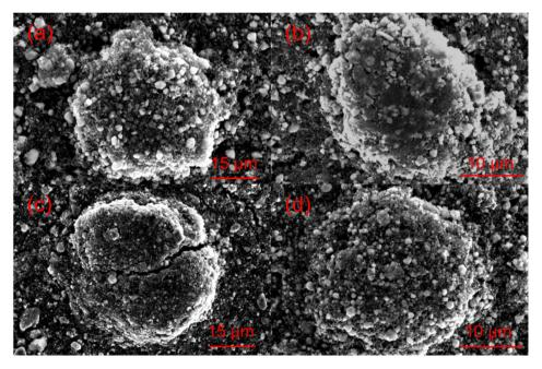
Fig. 11 SEM images of (a) pristine LiNiO<sub>2</sub>; (b) pristine Li<sub>1.1</sub>Ni<sub>0.85</sub>S<sub>0.05</sub>O<sub>2-x</sub> (c) LiNiO<sub>2</sub> after 200 cycles. (d) Li<sub>1.1</sub>Ni<sub>0.85</sub>S<sub>0.05</sub>O<sub>2-x</sub> after 200 cycles.
