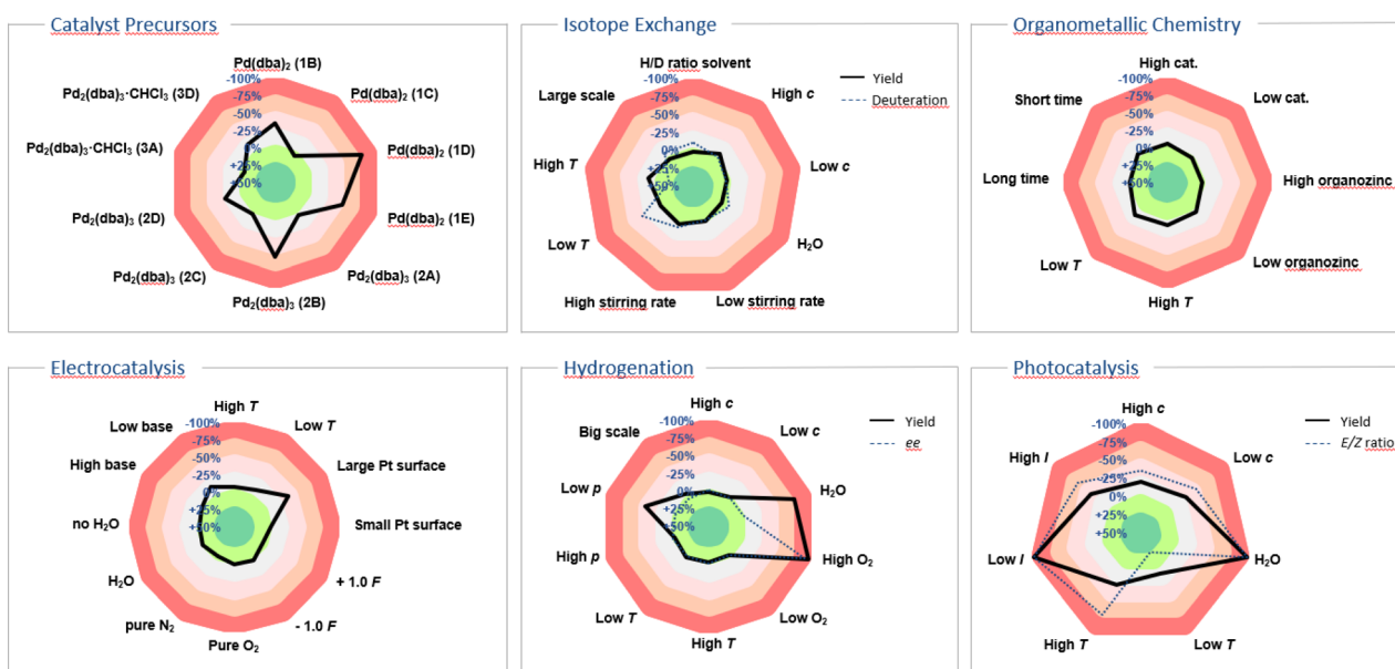
Fig. 2 Examples showcasing sensitivity screens tailored to diverse research fields. 13–16 In instances like hydrogenation, isotope exchange and photocatalysis the sensitivity screen was utilised to illustrate two target values, such as yield/deuterium incorporation, yield/enantiomeric excess and yield/ E:Z ratio, along with the parameters' impact on them.
