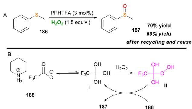
Scheme 43 (A) Activation of H<sub>2</sub>O<sub>2</sub> by an ionic liquid catalyst. (B) Proposed reaction mechanism.
