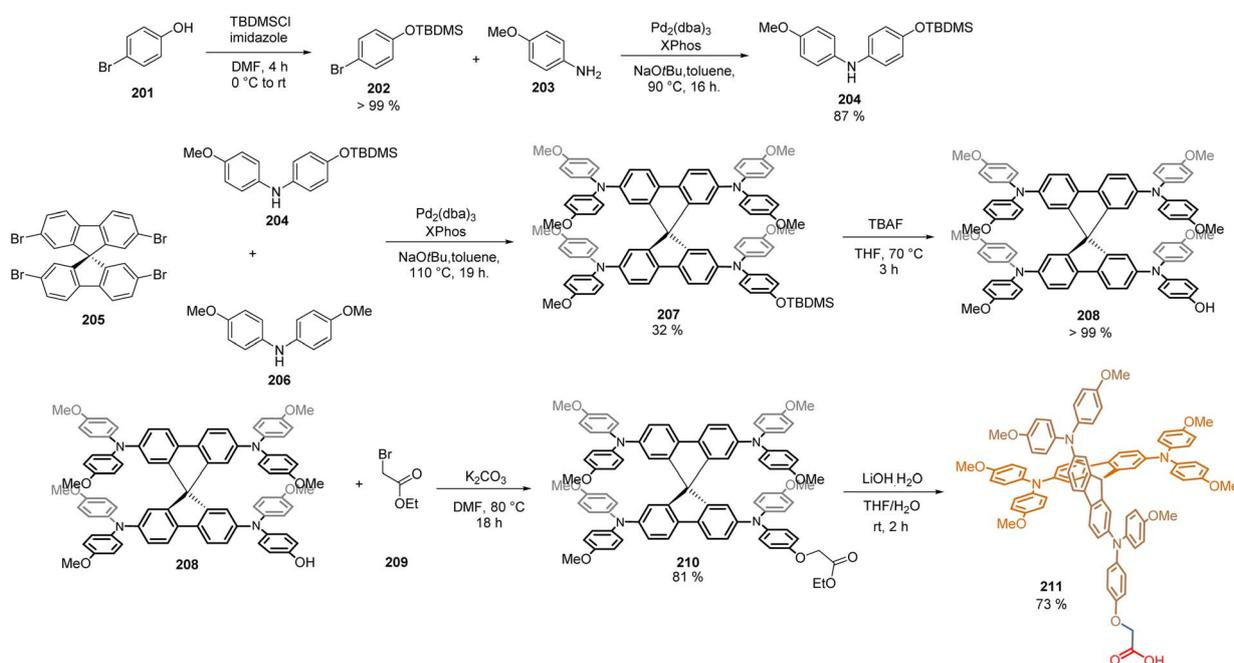
Scheme 32 Synthesis of the spiro OMeTAD derivative **211**.
