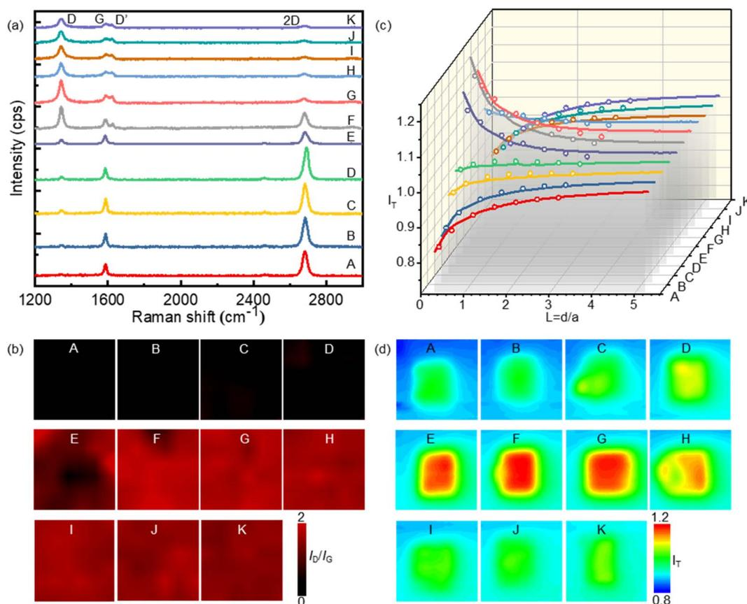
Fig. 2 (a) Raman spectra (vertically aligned) and (b) Raman  $I_{\text{D}}/I_{\text{G}}$  mapping of the brominated SLG patterns. (c) The probe approaching curves and (d) SECM images obtained on the brominated SLG patterns. In the SECM experiments, the tip electrode was held at a potential of 0.4 V in the electrolyte solution containing 1 mM FcMeOH and 0.1 M KCl, while the SLG substrate was kept unbiased. The tip–substrate distance was kept constant at  $2.2\ \mu\text{m}$  ( $d/a = 0.44$ ).
