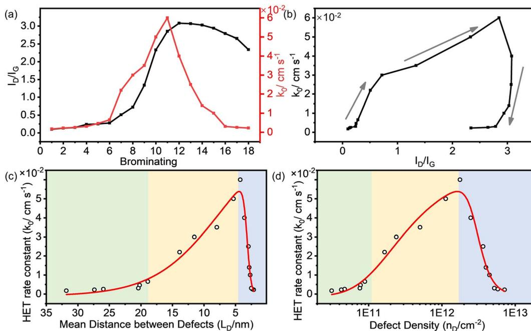
Fig. 3 (a) The  $I_D/I_G$  (black line) and the standard HET rate constant  $k^0$  (red line) varying with the continuation of the bromination process. (b) The correlation between  $I_D/I_G$  and  $k^0$ . (c and d)  $k^0$  as a function of defect density  $n_D$  ( $\text{cm}^{-2}$ ) and the mean distance between defects  $L_D$  (nm), respectively.
