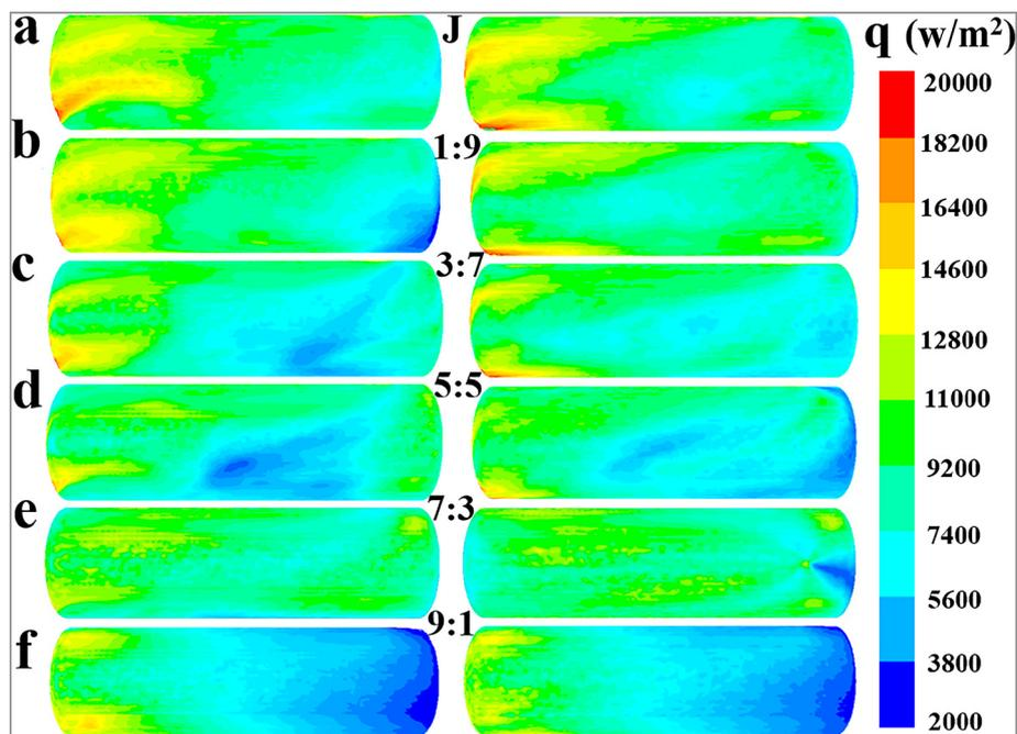
Fig. 5 Effect of flow ratios on the mean surface heat flux distribution characteristics of the jacket at the values of  $Q_1:Q_2$ : (a) J, (b) 1:9, (c) 3:7, (d) 5:5, (e) 7:3 and (f) 9:1.
