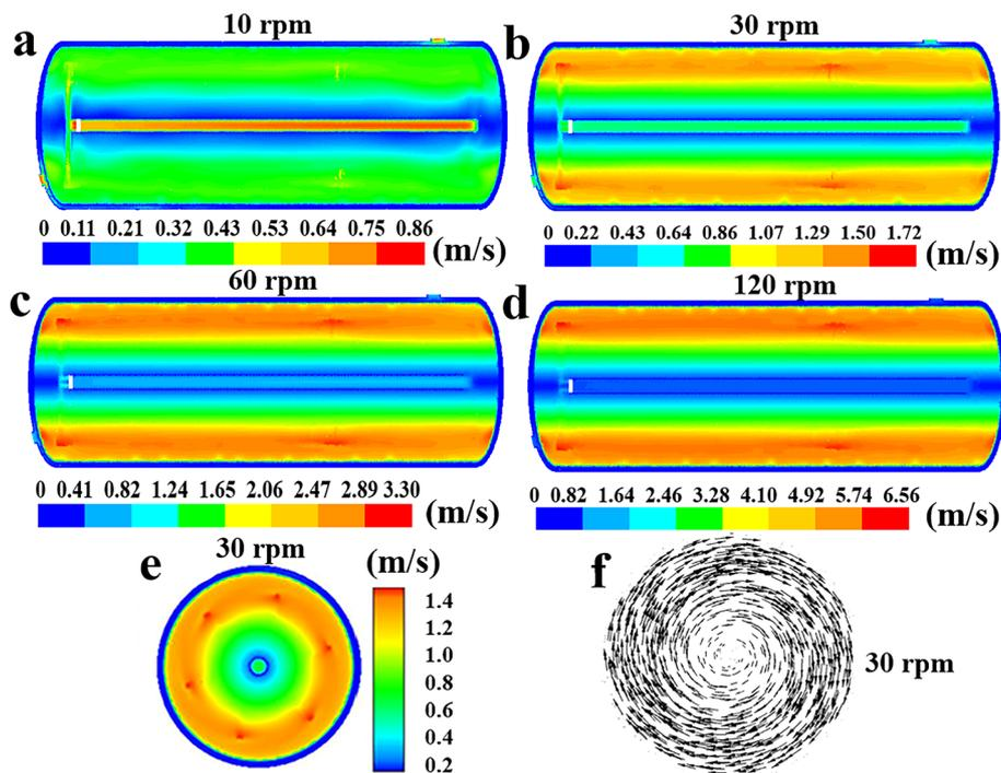
**Fig. 10** Effect of agitator speed on the distribution of fluid velocity along the reactor's axial cross section at  $n = 10$  rpm (a), 30 rpm (b), 60 rpm (c) or 120 rpm (d). (e) Fluid velocity and (f) velocity vector in the radial cross section at  $n = 30$  rpm.
