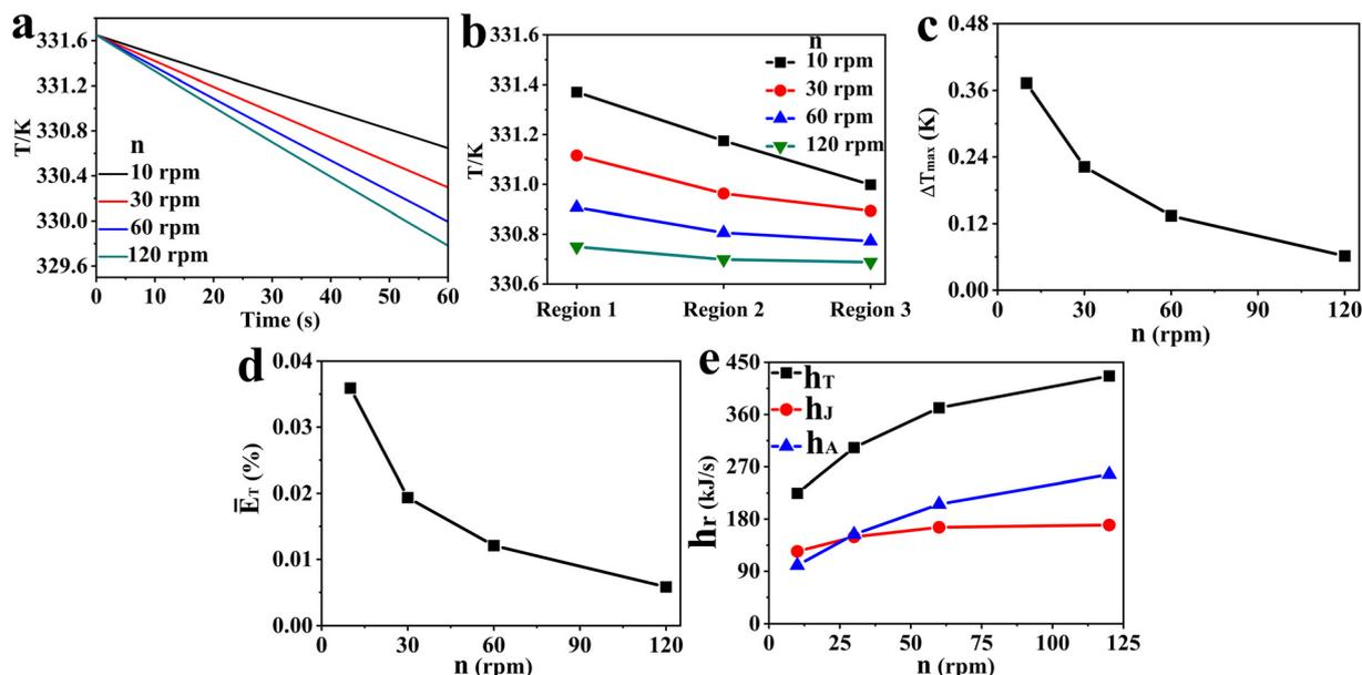
Fig. 8 Effect of agitator speeds on (a) fluid temperature in all reaction zones at different times, (b) average fluid temperature in various regions, (c)  $\Delta T_{\max}$ , (d)  $E_T$ , (e)  $h_T$ ,  $h_A$ ,  $h_J$ .
