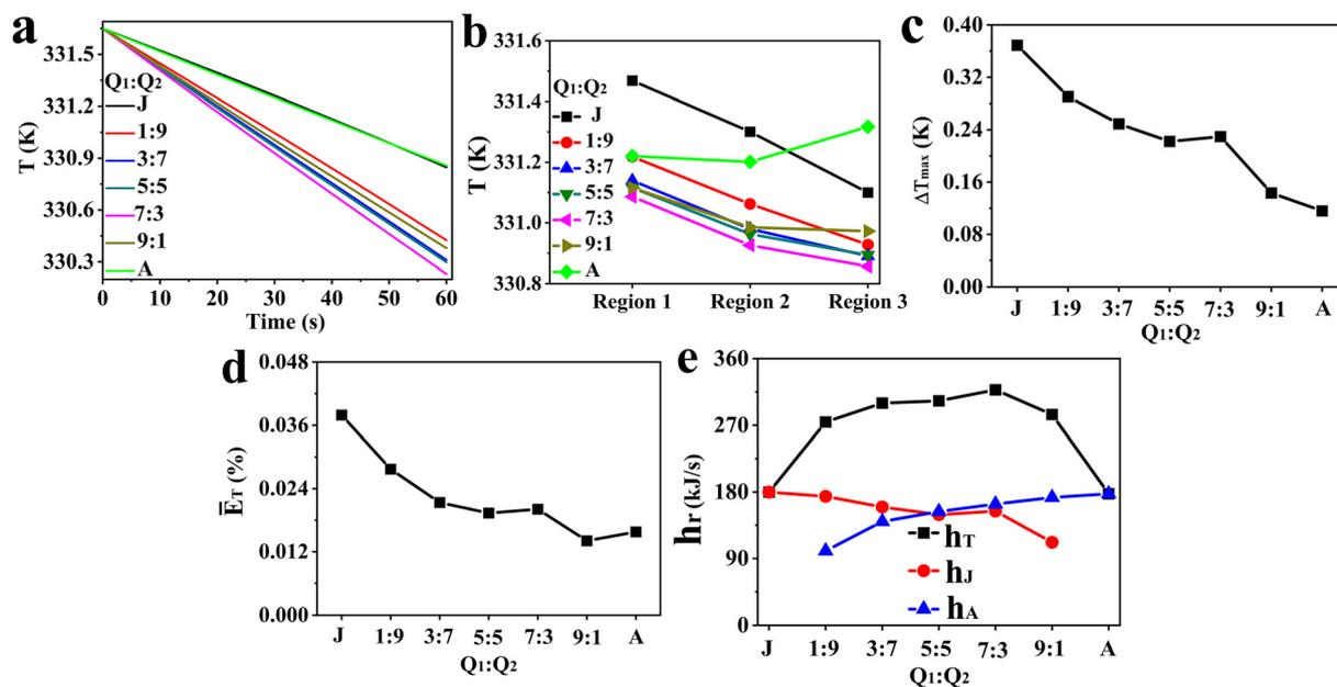
Fig. 4 Effect of  $Q_1:Q_2$  on (a) fluid temperature in the reaction zone at different times, (b) average fluid temperature in various regions, (c)  $\Delta T_{max}$ , (d)  $\bar{E}_r$ , and (e)  $h_T$ ,  $h_A$ ,  $h_J$  (J and A correspond to all cooling water entering the jacket and the agitator, respectively).
