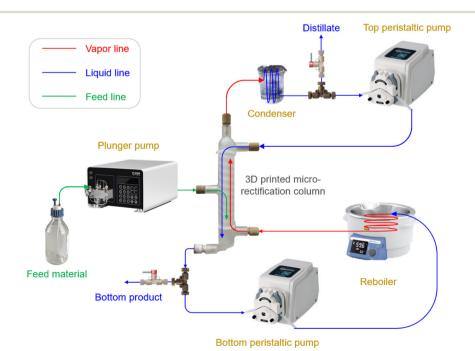
Fig. 1 Illustration of the experimental apparatus.
