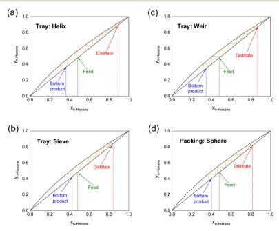
Fig. 3 McCabe-Thiele diagram of n-hexane/cyclohexane at total reflux ratio, with tray columns of (a) helix, (b) sieve, and (c) weir structures, and (d) the column with sphere packings. Conditions used in the experiments: 1 atm and 25 °C inlet temperature.
