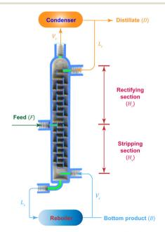
Fig. 5 1D mass transfer model of the microrectification geometry.
