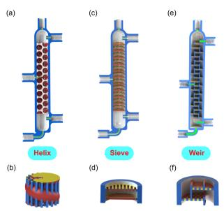
Fig. 2 Illustration of the tray columns, i.e., (a and b) helix, (c and d) sieve, and (e and f) weir structures. In order to better display the 3D structure, (b) shows the pathway through which the gas-liquid fluids flow, while (d) and (f) show half the structural units.
