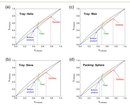
Fig. 4 McCabe-Thiele diagram of n-hexane/cyclohexane at a reflux ratio of 4.0, with tray columns of (a) helix, (b) sieve, and (c) weir structures, and (d) the column with sphere packings. The green, red, and blue solid lines denote the feed line, rectifying line, and stripping line, respectively. Conditions used in the experiments: 1 atm and 25 °C inlet temperature.
