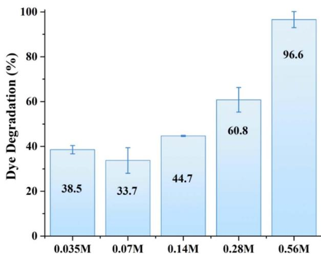
Fig. 3 MB dye photodegradation by various ZnO structures.
