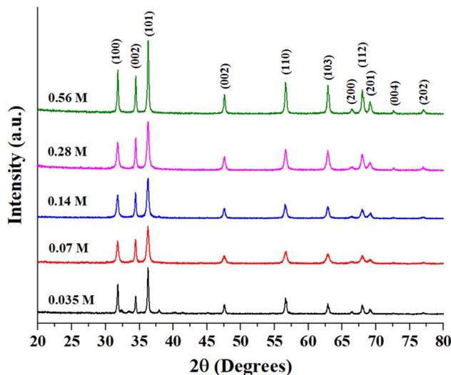
**Fig. 2** XRD patterns of as-prepared ZnO particles.
