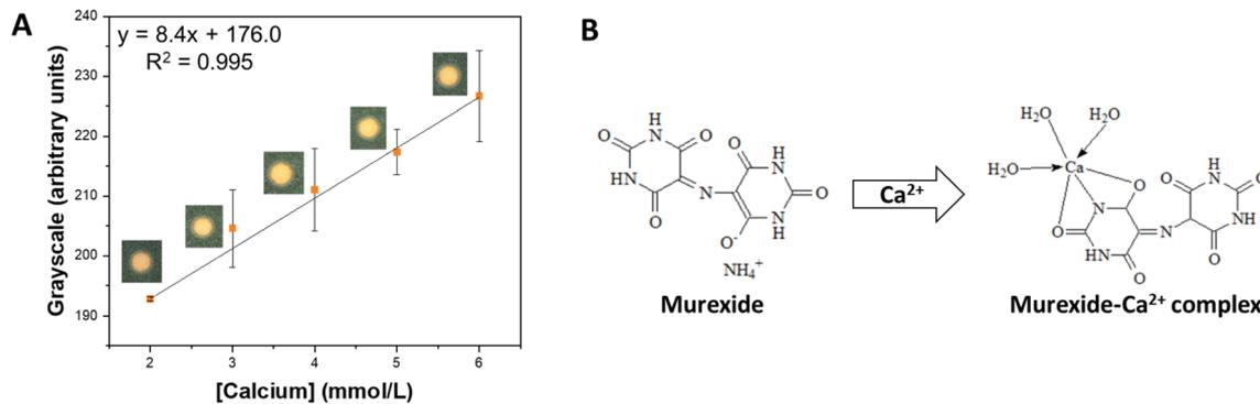
Fig. 3 Detection of calcium in the proposed  $\mu$ PAD. (A) Calibration curve obtained for  $\text{Ca}^{2+}$  in concentrations ranging from 2.0 to 6.0  $\text{mmol L}^{-1}$ . (B) Structure of murexide and the murexide- $\text{Ca}^{2+}$  complex.
