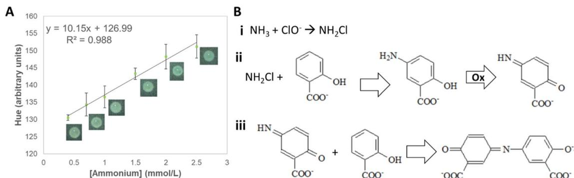
Fig. 5 Detection of ammonium in the proposed  $\mu$ PAD. (A) Calibration curve obtained for ammonium in concentrations ranging from 0.5 to 2.5  $\text{mmol L}^{-1}$ . (B) Reaction between (i) ammonium and hypochlorite, forming monochloramine; (ii) monochloramine and salicylate, forming 5-aminosalicylate and (iii) 5-aminosalicylate being oxidized in the presence of nitroprusside catalyst forming the blue colored indosalicylate compound.
