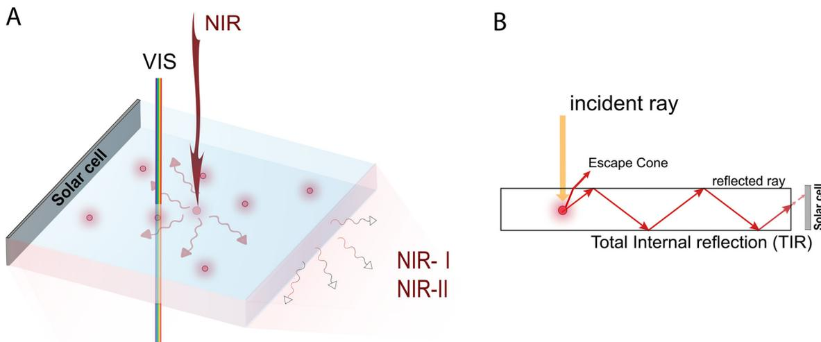
Fig. 1 (A) Sketch of a transparent LSC, (B) working principle of LSCs.
