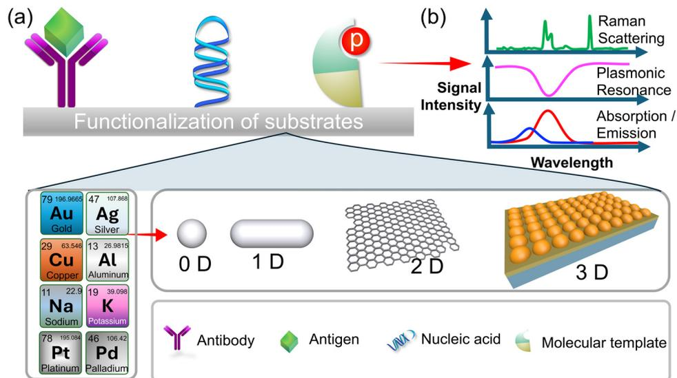
**Fig. 2** (a) The functionalization process of the substrate with various optical materials and the attachment of specific receptors for enhancement of sensitivity and specificity. (b) The signal detection mechanism, involving the selection of modes such as surface plasmon resonance (SPR), absorbance, transmission or Raman scattering, enabling precise analyte detection and analysis.<sup>93</sup>
