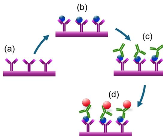
**Fig. 15** The schematic representation of the magneto-nanosensor biochip immunoassay involves several steps. (a and b) Immobilization of antibodies on the surface of the working electrode. (c) Sandwich structures are formed through the addition of biotinylated detection antibodies. (d) Magnetic nanoparticles bound to the detection antibodies generate a stray magnetic field that results in a change in sensor resistance due to the GMR effect.<sup>72</sup>
