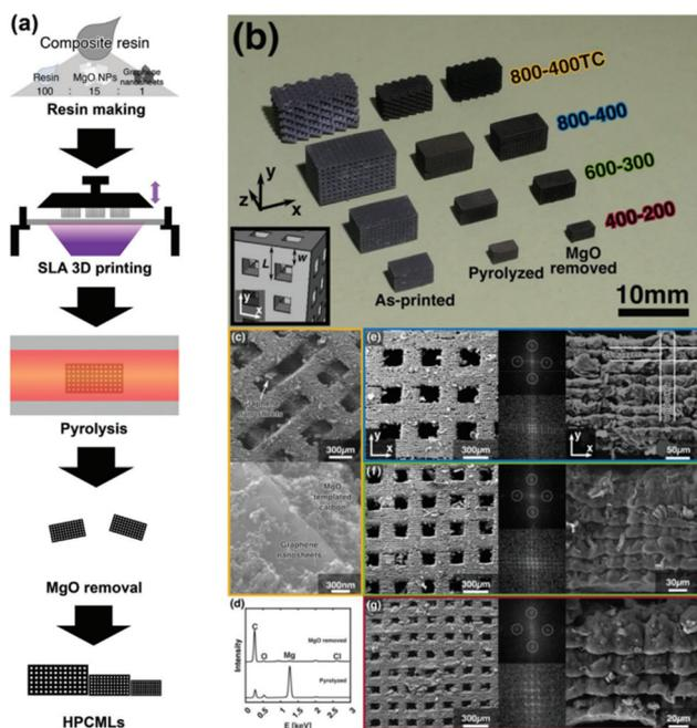
**Fig. 11** (a) Schematic process for the preparation of a hierarchical porous carbon microlattice by SLA; (b) an optical image of four types of samples at each step of preparation: as-printed, pyrolyzed, and MgO removed; (c) SEM images of sample 800–400°C with different magnifications; (e–g) SEM images with different magnifications and FFT patterns of the other three types of samples.<sup>83</sup>
