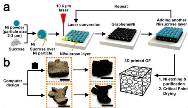
Fig. 14 Schematic of *in situ* synthesis of 3D graphene foam using SLS.<sup>94</sup>
