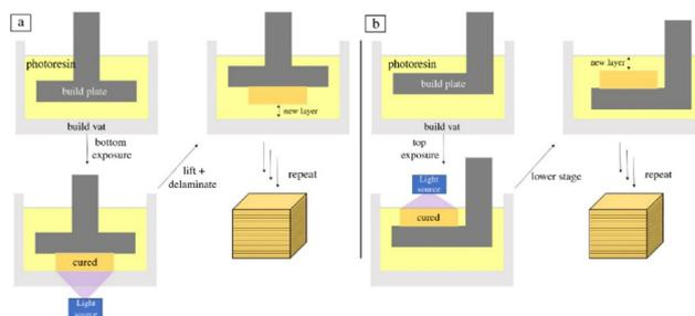
Fig. 3 Schematic of layer-based vat photopolymerization where the light is oriented from (a) the bottom and (b) the top.<sup>52</sup>
