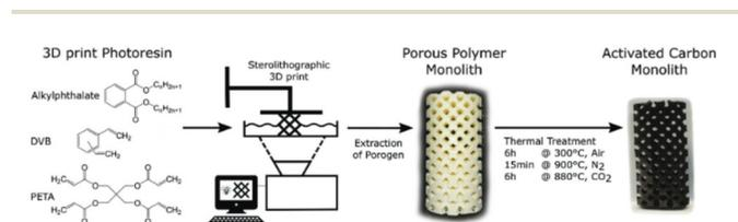
Fig. 8 Schematic overview of the SLA printing process to produce porous carbon.<sup>79</sup>
