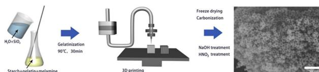
Fig. 5 Schematic illustration of the DIW process to produce porous carbon.<sup>68</sup>
