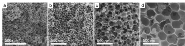
**Fig. 6** SEM of the printed carbon replicas with different  $\text{SiO}_2$  diameters: (a) 50 nm; (b) 100 nm; (c) 200 nm; and (d) 350 nm.<sup>69</sup>
