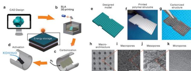
Fig. 9 Schematic of the SLA print process and SEM/TEM imaging of macroarchitectures, macropores, mesopores, and micropores with scale bars of 1 mm, 20  $\mu\text{m}$ , 100 nm, and 5 nm, respectively.<sup>80</sup>
