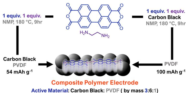
**Fig. 6** Comparative approach to generate composite polymer electrodes where polymerization is done either separate from or in the presence of conductive carbon additive. Polymerizing in the presence of carbon additive leads to higher measured capacities at fast charge/discharge rates. Adapted with permissions from ref. 40. Copyright © 2018 Royal Society of Chemistry.
