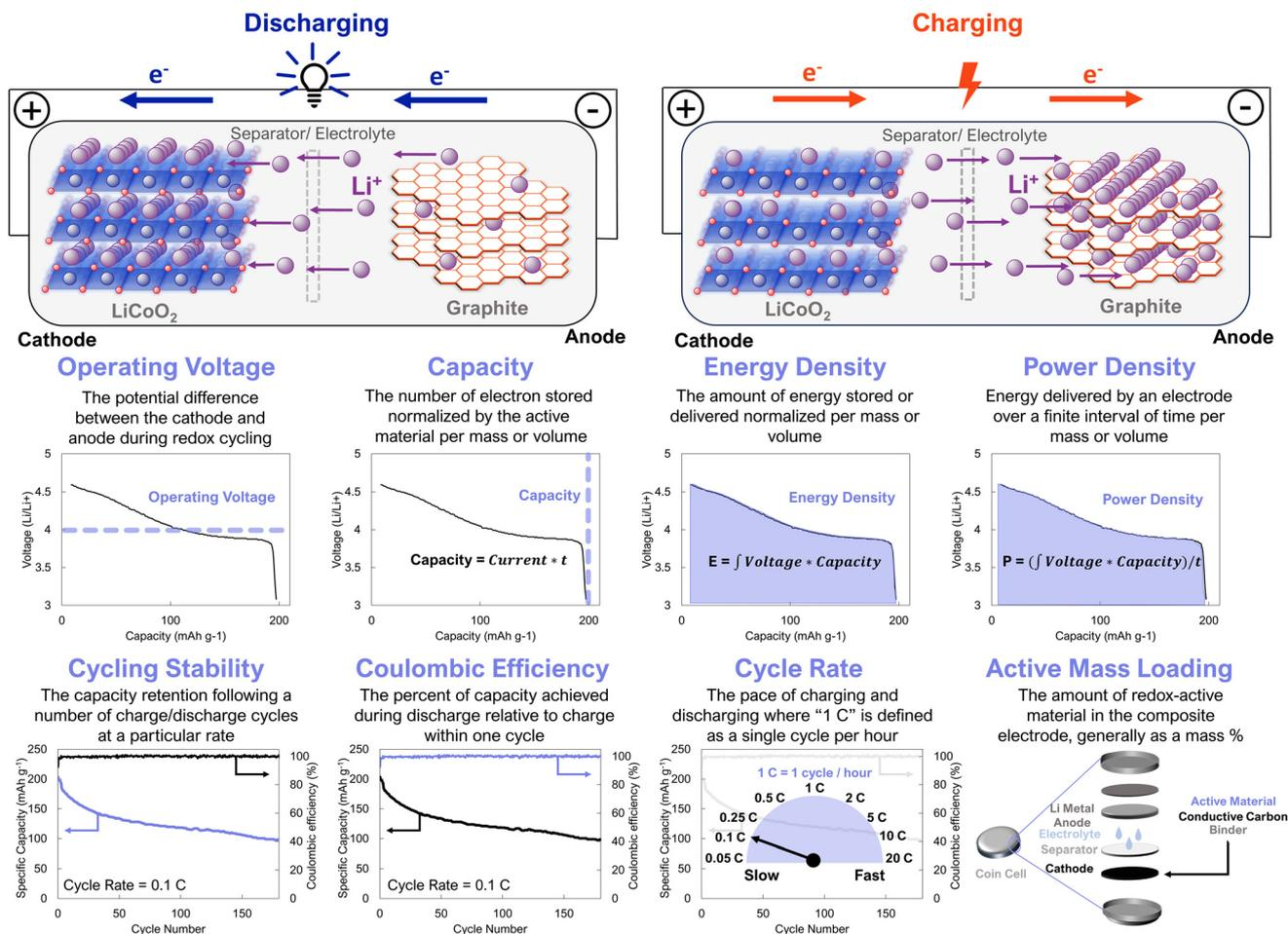
**Fig. 1** Schematic of battery charging/discharging processes and common performance metrics to evaluate new electrode active materials. Data is for LiCoO<sub>2</sub>, which was adapted with permissions from ref. 5. Copyright © 2022 Wiley.
