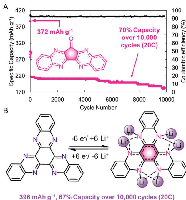
**Fig. 9** (A). Performance of a quinoxaline-based cathode at a 20C rate. (B). Structure of a quinoxaline-based electrode in its fully lithiated state. Adapted with permissions from ref. 56. Copyright © 2017 Springer Nature Limited.
