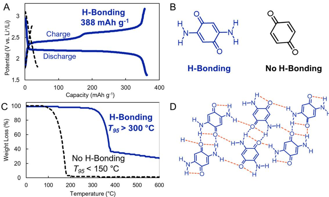
**Fig. 8** (A). Electrochemical cycling of (B). molecular electrodes that host (blue) or do not host (black) hydrogen bonding interactions. (C). Thermogravimetric analysis (TGA) the electrodes. (D). Supramolecular interactions present in electrode hosting H-bonding interactions (2,5-diamino-1,4-benzoquinone). Adapted with permissions from ref. 51. Copyright © 2018 Royal Society of Chemistry.
