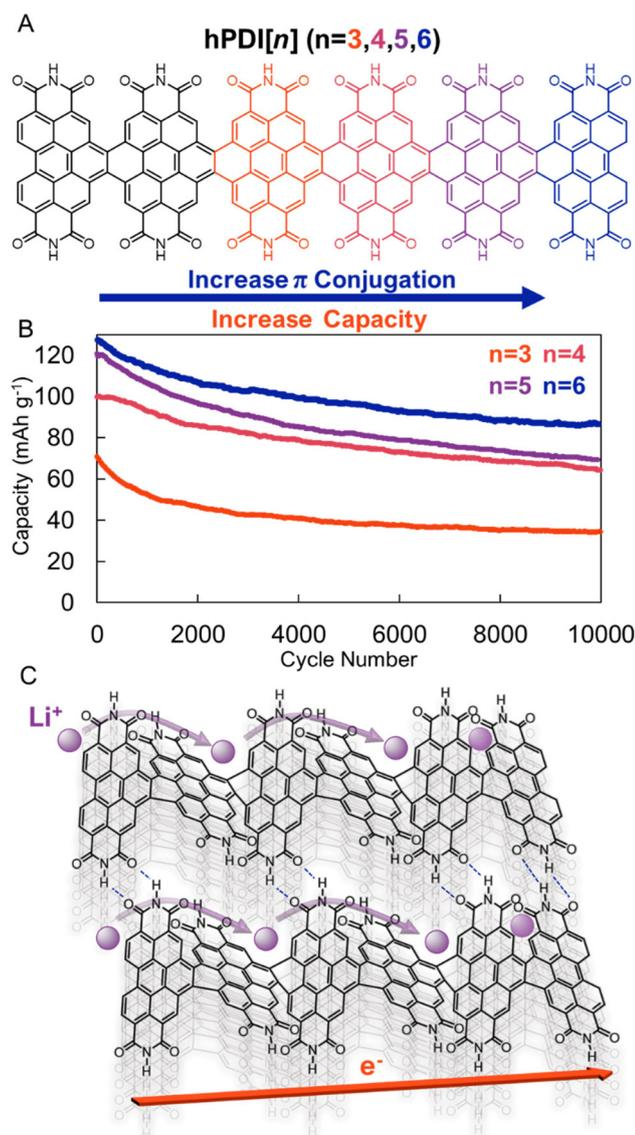
**Fig. 5** (A). Helical PDI nanoribbons (hPDI[n]). (B). Cycling performance of hPDI[n]-based electrodes at 7.7C over 10 000 cycles. (C). Graphical depiction of contorted PDI nanoribbon with high ionic and electronic conductivities. Adapted with permissions from ref. 39. Copyright © 2022 American Chemical Society.
