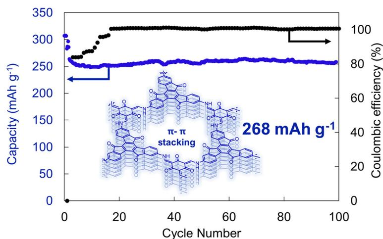
**Fig. 7** Electrochemical cycling of a truxenone-based 2D polymer at 0.1C rate. Structure depicted showcases the  $\pi$ - $\pi$  interactions between the different layers of the 2D polymer. Adapted with permissions from ref. 41. Copyright © 2020 Wiley Online Library.
