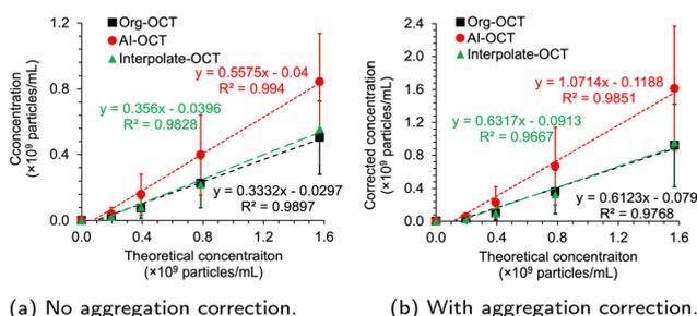
**Fig. 3** Correlation of OCT-based particle concentrations with theoretical concentrations and dilutions. The regression line was obtained without the 800× diluted sample. (a) No aggregation correction. (b) With aggregation correction.
