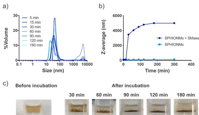
**Fig. 2** *In vitro* degradation of SPHIONMs by SMase. (a) Changes in the hydrodynamic size distribution of the SPHIONM solution incubated with sphingomyelinase from  $t = 5$  to  $t = 180$  min. (b) Changes in z-average of SPHIONM solutions incubated with or without sphingomyelinase from  $t = 5$  to  $t = 180$  min. The experiments were performed at 37 °C in PBS and were repeated twice. (c) Visual evaluation of SPHIONMs aggregation after incubation with sphingomyelinase.
