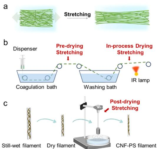
**Fig. 9** Schematic presentation of (a) CNF network changes practically the CNF orientation during the wet stretching process, (b) pre-drying and in-process stretching processes and the (c) post-drying stretching process.<sup>51</sup> Adapted with permission from ref. 51. Copyright 2023 Elsevier.
