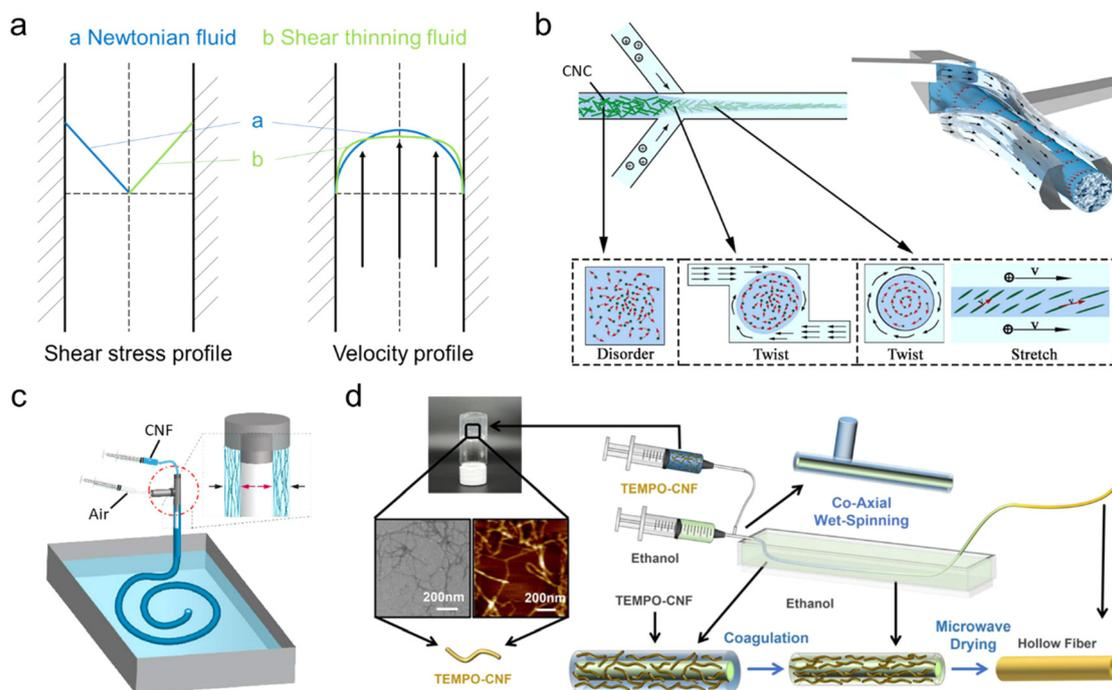
**Fig. 7** (a) Estimated shear stress profile and velocity profile within the spinning spinneret. Schematic presentation of special wet spinning spinnerets: (b) convection focusing device.<sup>70</sup> Adapted with permission from ref. 70. Copyright 2018 Elsevier. (c) Coaxial spinning device with compressed air as the inner flow.<sup>91</sup> (d) Coaxial spinning device with coagulation batch as the inner flow.<sup>125</sup> Adapted with permission from ref. 125. Copyright 2023 ACS.
