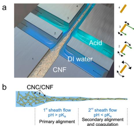
**Fig. 6** (a) Schematic of a typical flow-focusing device with double channels used for CNF assembly.<sup>67</sup> (b) The schematic presentation of nanocellulose orientation and gelation in the microfluidic device.<sup>71</sup> Adapted with permission from ref. 71. Copyright 2019 Wiley.
