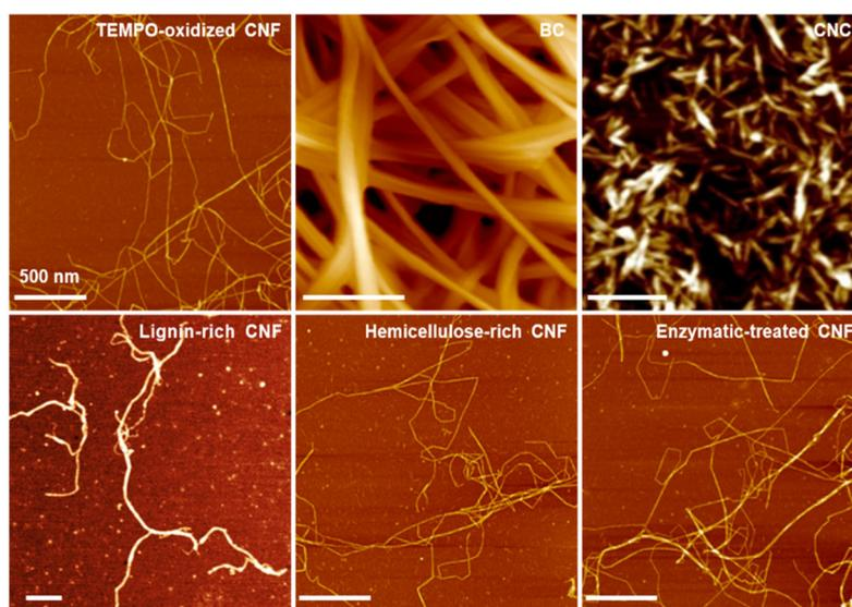
**Fig. 2** AFM images of different types of nanocelluloses. Adapted with permission from ref. 122 and 123. Copyright 2021, 2019 Springer Nature.<sup>82,122–124</sup>
