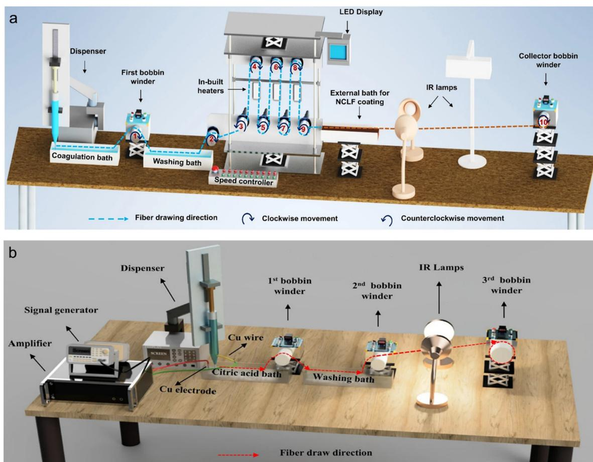
**Fig. 11** The representative schematic diagrams of the integrated wet spinning device for the continuous fabrication of CNF wet-spun fibers with (a) in-built heaters<sup>61</sup> and (b) AC electric field.<sup>105</sup> Adapted with permission from ref. 61 and 105. Copyright 2022, 2023 Springer Nature.
