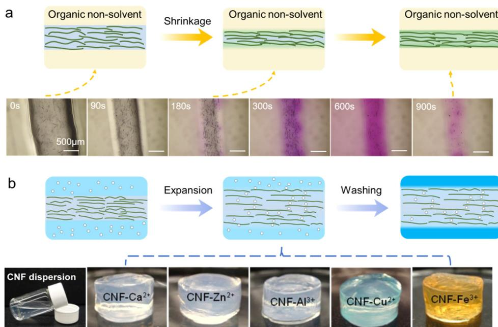
**Fig. 8** Schematic presentations of the coagulation process using different coagulation baths and the corresponding still-wet fibers: (a) organic non-solvents.<sup>51</sup> Adapted with permission from ref. 51. Copyright 2023 Elsevier. (b) Ion solutions containing acids or salts.<sup>126</sup> Adapted with permission from ref. 126. Copyright 2013 ACS.
