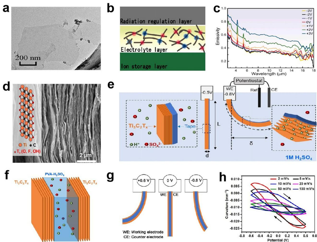
**Fig. 14** (a) HRTEM image of MXene nanosheets. (b) Structure and (c) emissivity of the MXene-based EC device. (a–c) Adapted with permission from ref. 83. Copyright 2022, Elsevier. (d) Cross-sectional SEM image of a  $\text{Ti}_3\text{C}_2\text{T}_x$  electrode. (e) Schematic representation of the EC film. (f and g) The configuration and (h) curvature of the EC actuator. (d–h) Adapted with permission from ref. 84. Copyright 2019, American Chemical Society.
