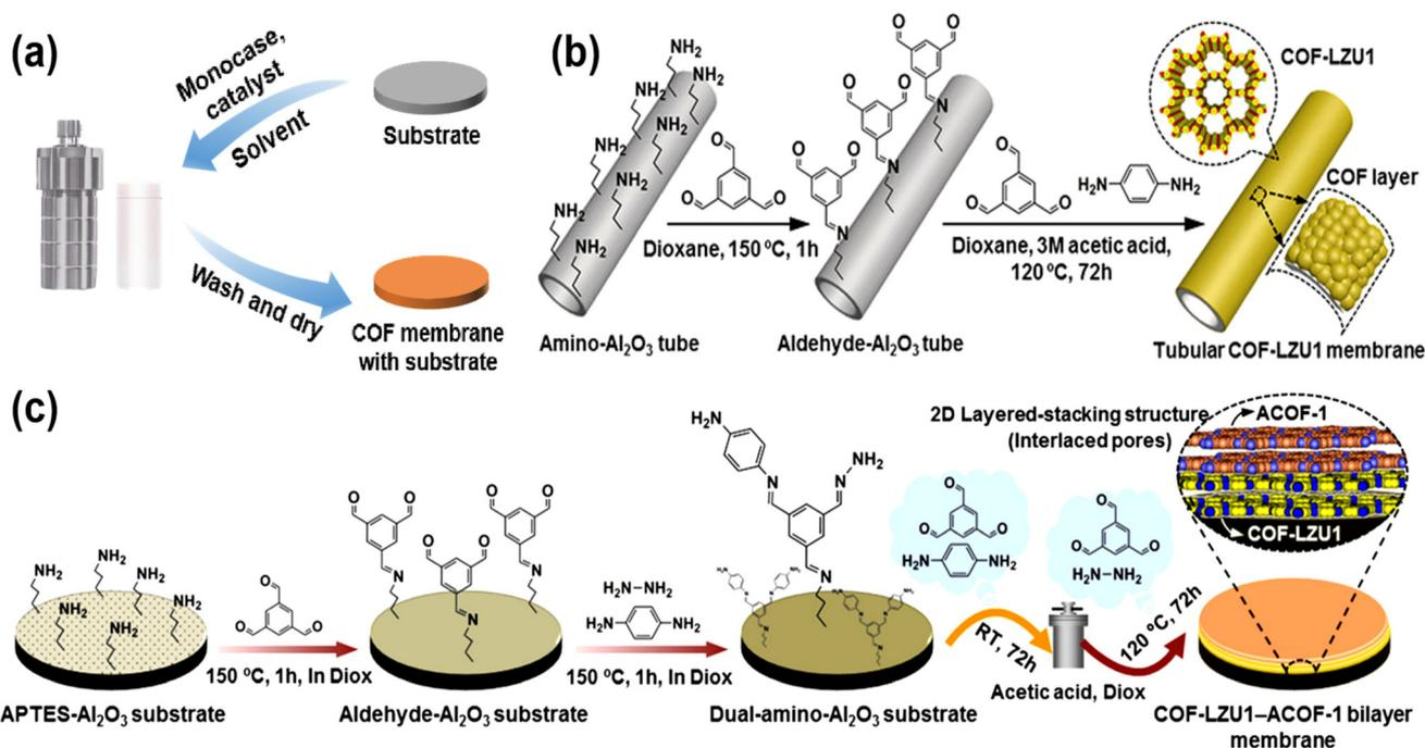
**Fig. 3** (a) The general process of preparing COF membranes by the solvothermal method. (b) Synthesis of tubular COF-LZU1 membranes. Reproduced with permission from ref. 33. Copyright 2018, Wiley-VCH Verlag GmbH & Co. KGaA, Weinheim. (c) Schematic representation of the synthesis of a COF-LZU1-ACOF-1 bilayer membrane by a temperature-swung solvothermal approach. Reproduced with permission from ref. 34. Copyright 2018, American Chemical Society.
