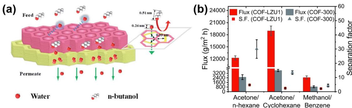
**Fig. 12** (a) Yang<sup>53</sup> et al.'s design of a bilayer COF membrane with 0.39 nm pores for the separation of water and *n*-butanol. Reproduced with permission from ref. 53. Copyright 2020, Royal Society of Chemistry. (b) The flux and separation factor of COF membranes (COF-LZU1 and COF-300). Reproduced with permission from ref. 120. Copyright 2023, the Authors. Published by Elsevier B.V.
