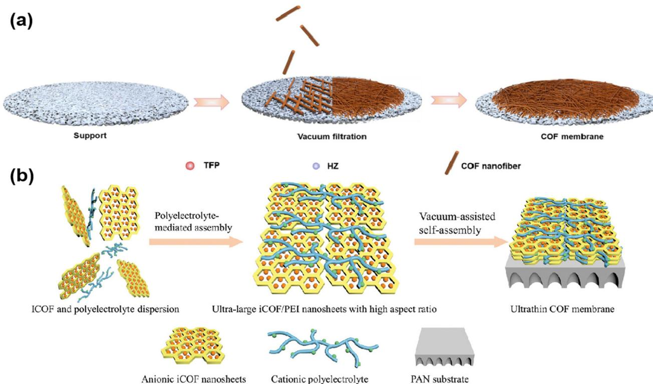
**Fig. 6** (a) The formation process of the TpHZ COF membrane. Reproduced with permission from ref. 21. Copyright 2023, Elsevier B.V. (b) Illustration of a polyelectrolyte-mediated assembly strategy to prepare ultrathin COF membranes. Reproduced with permission from ref. 71. Copyright 2023, Wiley-VCH GmbH.
