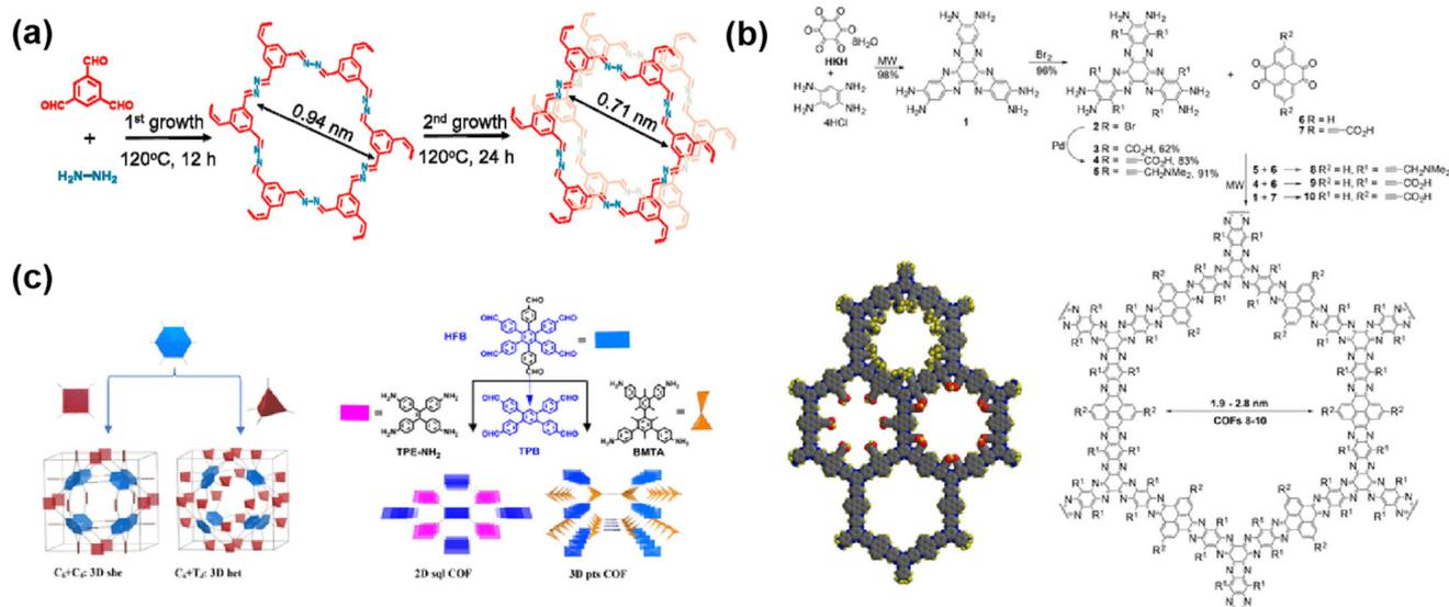
**Fig. 7** (a) Aperture changes in COF after primary and secondary growth. Reproduced with permission from ref. 79. Copyright 2021, Elsevier. (b) Synthesis process and pore size of COF 8–10. Reproduced with permission from ref. 82. Copyright 2018, American Chemical Society. (c) Design and synthesis of three-dimensional mesh COF. Reproduced with permission from ref. 81. Copyright 2021, American Chemical Society.
