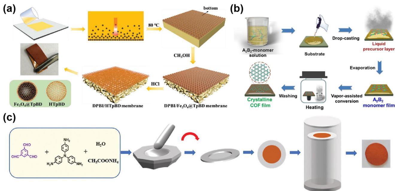
**Fig. 5** (a) The proposed preparation process of DPBI/HTpBD composite membranes. Reproduced with permission from ref. 63. Copyright 2022, Wiley-VCH GmbH. (b) The preparation of crystalline COF film by the vapor-assisted conversion method. Reproduced with permission from ref. 59. Copyright 2021, Chinese Chemical Society. (c) Reproduced with permission from ref. 65. Copyright 2023, Wiley-VCH GmbH.
