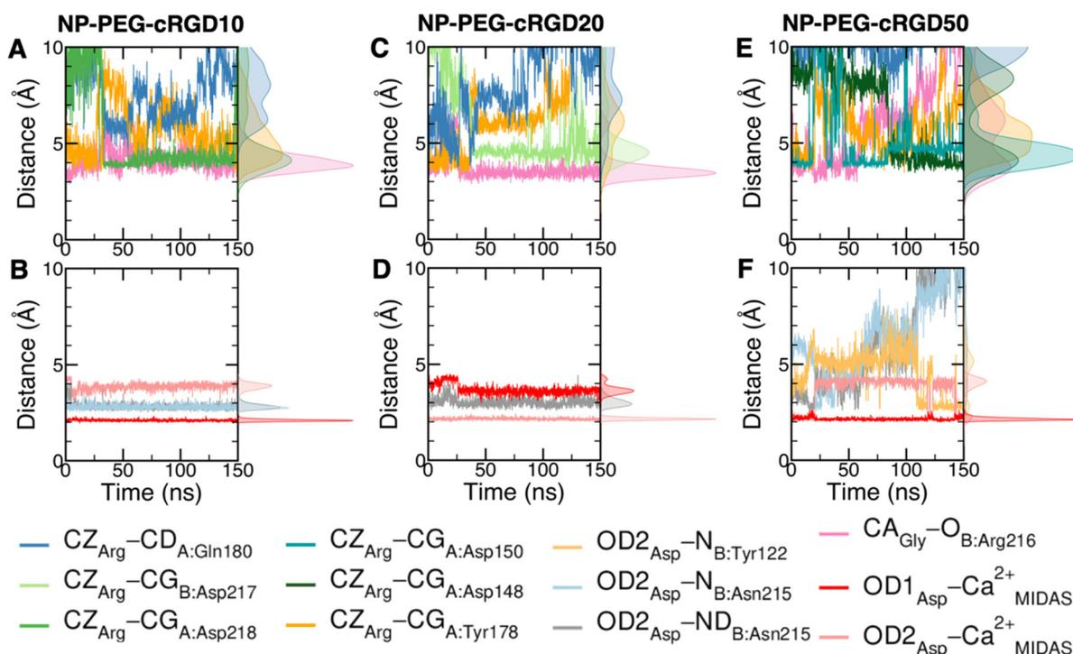
**Fig. 6** Distances values and histograms between CZ of arginine, CA of glycine and OD1 and OD2 of aspartate and the protein atoms they are interacting with along the *NP-cRGD MD simulations* at the lowest (A and B), intermediate (C and D) and highest (E and F) cRGD density. Only relevant interactions are reported for each simulation.
