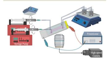
Fig. 3 A schematic of the experimental setup including the μ-EFC, syringe pump with in-syringe mixing, an inverted microscope, a highspeed camera, a potentiostat, and outlet reservoirs.
