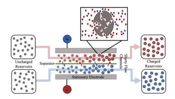
**Fig. 1** EFC schematic demonstrating the main components of the traditional EFC architecture: stationary electrodes, flow channels, an ion-exchange membrane separator, and slurry reservoirs. The zoomed-in particle view shows the EDL formation in the pores of the activated carbons.
