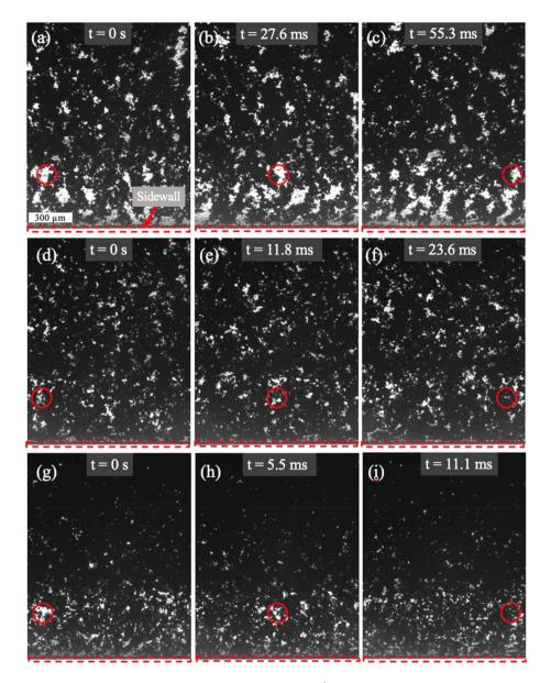
Fig. 5 Images from high-speed videos at (a-c) 35, (d-f) 50, and (g-i) 100  $\mu$ L min<sup>-1</sup> at 10× magnification with the channel sidewall at the bottom of each image, as denoted by the dashed red lines. The red circles track a void space across the width of the view field. The scale bar in (a) also applies to (b-i) and represents 300 µm.
