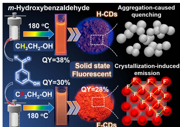
Fig. 1 Schematic of the synthesis procedures; optical images of the CDs dispersed in ethanol solution under 365 nm UV light. Schematic diagram of the SSF mechanism model.
