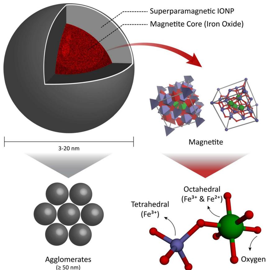
Fig. 6 (a) Superparamagnetic iron oxide nanoparticles (SPIONs). (b) Face-centered cubic (FCC) closed packing, with  $\text{Fe}^{3+}$  in the tetrahedral sites and  $\text{Fe}^{2+}$  occupying the octahedral sites.
