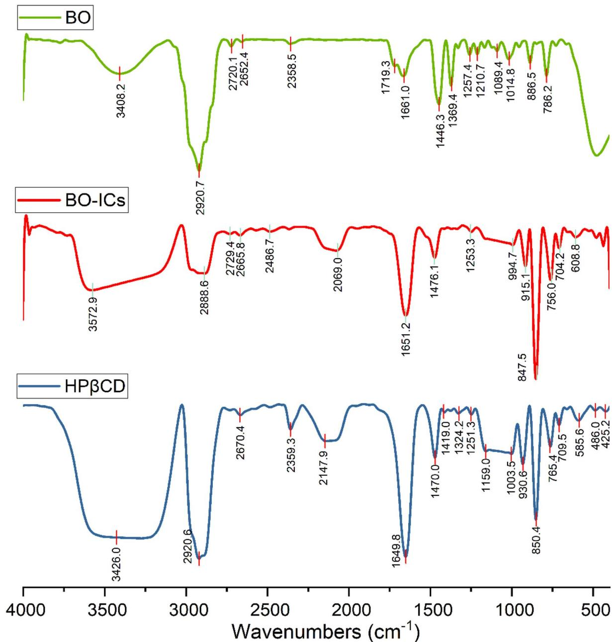
Fig. 3 FTIR spectra of BO, BO-ICs, and HPβCD.
