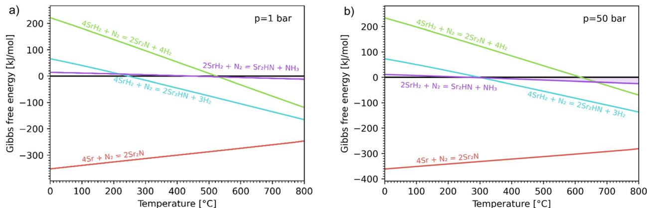
Fig. 3 Ellingham diagram of the nitridation step for reactions (3)–(6). Variation of the Gibbs free energy change per mol N<sub>2</sub> as a function of temperature for (a) standard  $\Delta G_{\text{rxn}}^\circ$ ; and (b)  $\Delta G_{\text{rxn}}$  at 50 bar assuming 20% reaction extent.
