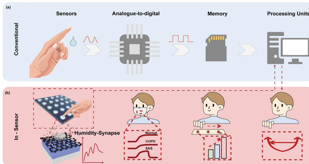
**Fig. 1** (a) The architecture of conventional sensors. Sensor outputs (analog signals) are first converted into digital signals (generated by an ADC chip) and stored in memory. The processing unit loads the data from the memory, and then transfers output signals back to the memory for storage. (b) The architecture of in-sensor computing with both sensing and storage capabilities; data can be transmitted directly to the processing unit, eliminating intermediate redundant steps.
